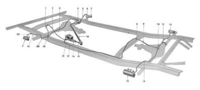
2. Brake Tube - Master Cylinder to Front Hose 3. Brake Tube - Tee to Front Brake Hose, Right 4. Brake Pedal 5. Brake Hose - Front Axle 6. Brake Tube - Wheel Cylinder to Hose 7. Wheel Brake Cylinder -Front 8. Brake Hose Spring Lock Clip 9. Brake Hose Assembly 10. Rear Brake Tee 11. Brake Tube - Rear Axle
